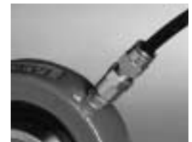
5. And plug the tube into the Quicklinc adapter
