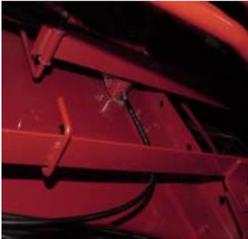
Install one # 244055 fitting, replacing grease zerk for Unloader Drive Tightener Arm. Route/install tubing from **Outlet 1** of valve.
