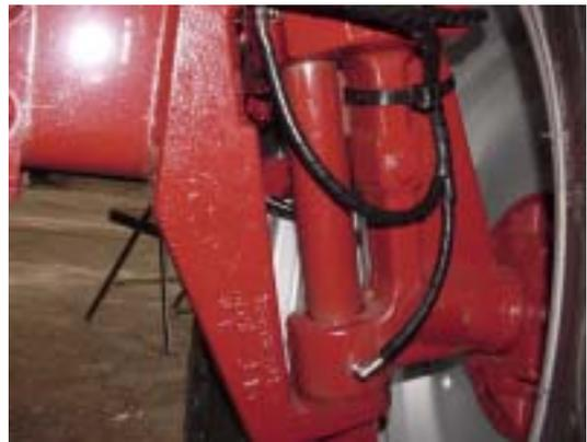
Install one # 244048 or 244047 and 20026 fittings, replacing grease zerk from Steering Knuckle Right Lower. This may require drilling and tapping to 1/8" NPT. Route/install tubing from **Outlet 5** of Rear Axle Valve.
