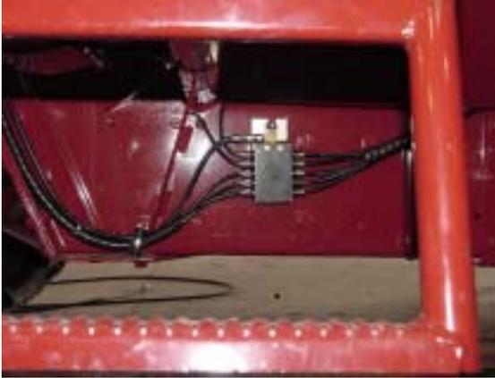
Mount **Right Rear Secondary Valve** and bracket as shown above.
