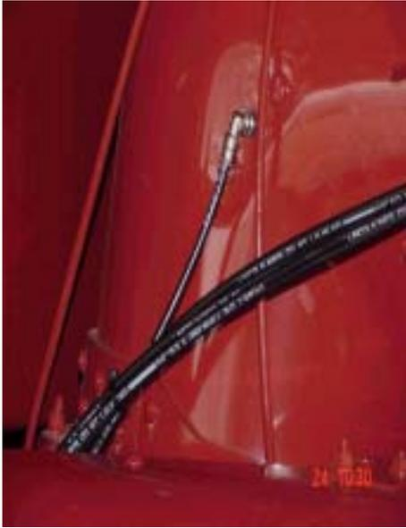
**2002 and prior.** Install one of #244054 Fitting, replacing grease zerk or Unloader Auger Upper Elbow Gearbox. Route/install tubing from **Outlet 10** of valve.
