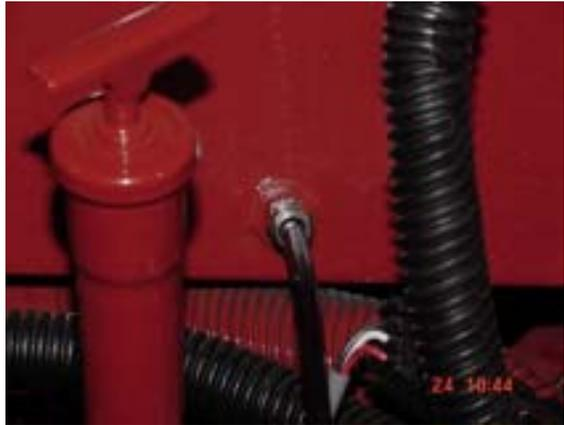
Install one # 244055 Fitting, replacing grease zerk for Feeder and Cleaning Fan Gear Case. Route/install tubing from **Outlet 3** of Right Front Valve.
