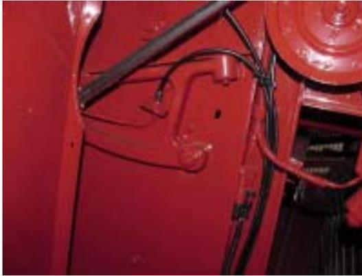
Install one # 244055 Fitting, replacing grease zerk for Chaffer Hanger. Route/install tubing from **Outlet 8** of Right Rear Valve.
