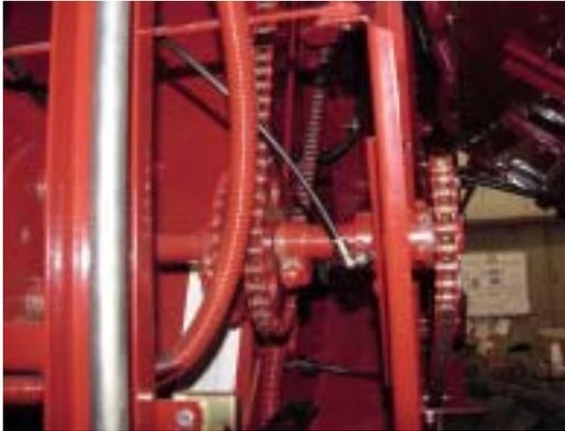
Install one of 270784 Zerk-Lock and # 243699 Swivel Fitting, replacing grease zerk for Elevator Outer Shaft Bearing. Route/install tubing from **Outlet 2** of Right Rear Valve.
