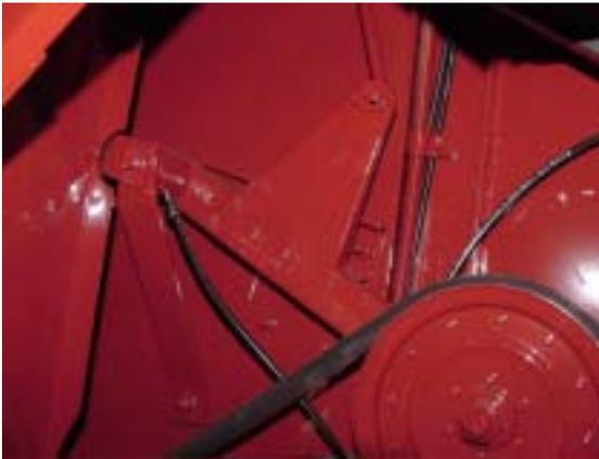
Install one # 244055 fitting, replacing grease zerk for Fan Driven Pulley. Route/install tubing from **Outlet 10** of Right Rear Valve.
