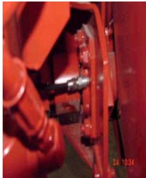
Install one # 244055 fitting, replacing grease zerk for Feeder Shaft Bearing. Route tubing from **Outlet 6** of valve.
