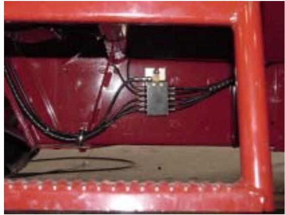
Install hose from **Outlet 12** of Primary Valve into inlet of Right Rear Secondary Valve.
