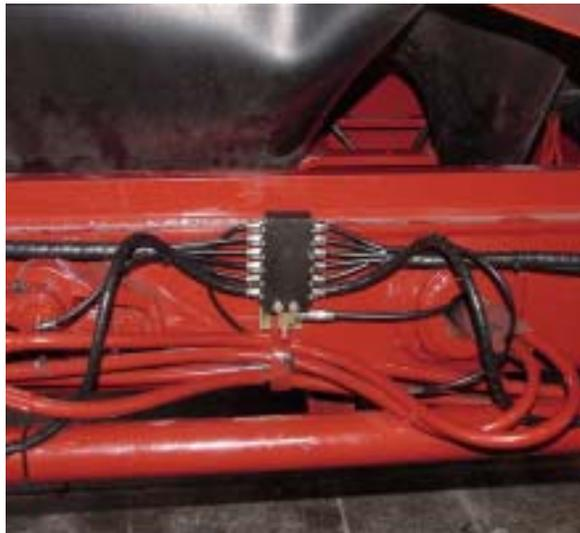
Install hose from **Outlet 1** of Primary Valve into inlet of Rear Axle Secondary Valve.
