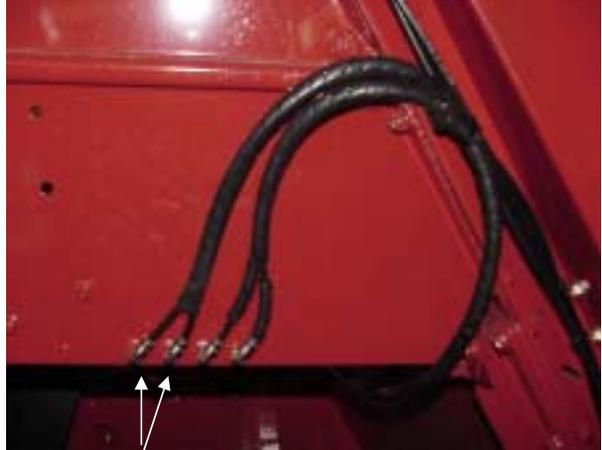
Install two # 244054 fittings, replacing grease zerks from Steering Axle Pivot Rear Upper and Lower. Route/install tubing from **Outlets 1 and 2** of Rear Axle Valve.
