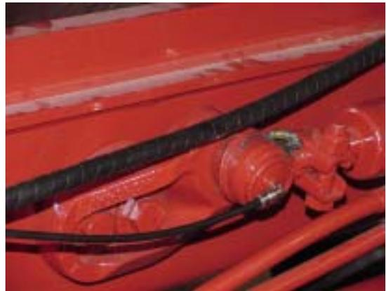
Install one # 244054 fitting, replacing grease zerk from Steering Cylinder Right. Route/install tubing from **Outlet 9** of Rear Axle Valve.
