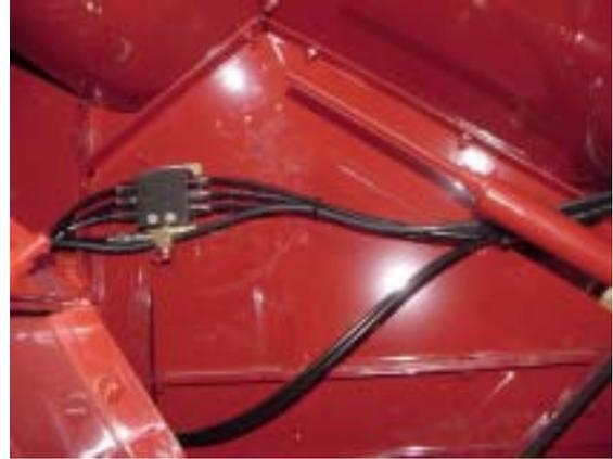
Mount **Right Front Secondary Valve** and bracket behind right front wheel.
