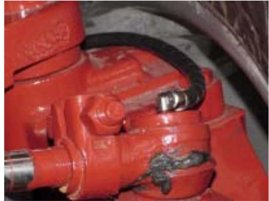
Install one 244054 fitting, replacing grease zerk from Steering Cylinder Ball Joint Right. Route/install tubing from **Outlet 7** of Rear Axle Valve.
