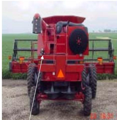
Mount the QLS-401 pump to pump mounting bracket, using hardware supplied in the pump box. Mount pump and bracket to the deck with two 247023 bolts. To accomplish this, you will need to drill two holes through the rear deck to the left of the walkway and just outside the hand rail. This pump incorporates the primary valve that will feed all the secondary valves, that in turn supply the lubrication points.
