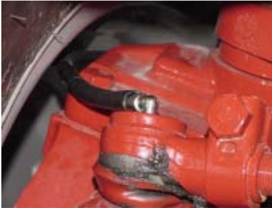
Install one 244054 fitting, replacing grease zerk from Steering Cylinder Ball Joint Left. Route/install tubing from **Outlet 8** of Rear Axle Valve.
