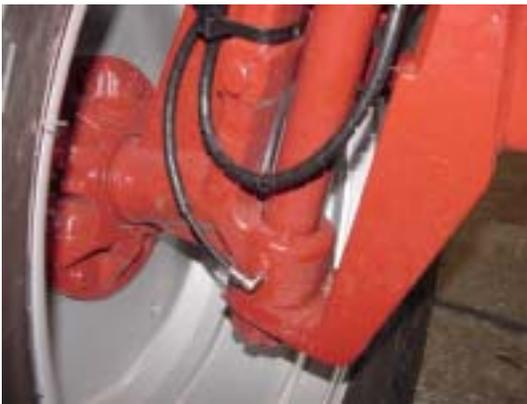
Install one # 244048 or 244047 and 20026 fittings, replacing grease zerk from Steering Knuckle Left Lower. This may require drilling and tapping to 1/8" NPT. Route/install tubing from **Outlet 6** of Rear Axle Valve.
