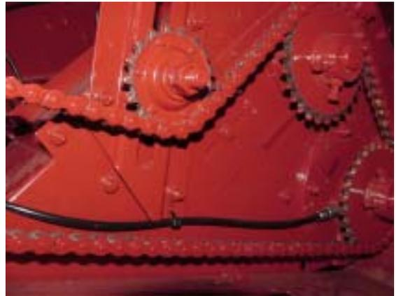
Install one # 270784 Zerk-lock adapter and # 244047 fitting, replacing grease zerk for Tailings Auger Shaft Bearing. Route/install tubing from **Outlet 7** of Right Rear Valve.
