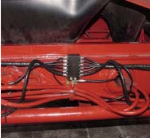
Mount Rear Axle Secondary Valve and valve bracket on beam over tie-rod.
