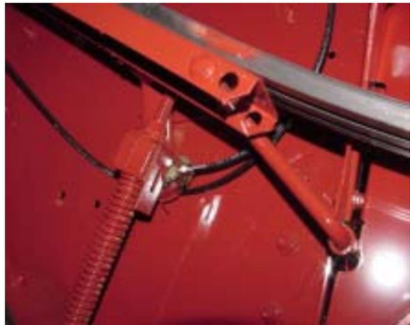
Install one # 244055 Fitting, replacing grease zerk for Tailings Delivery Auger. Route/install tubing from **Outlet 1** of Right Front Valve.
