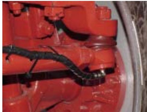
Install one of 244054 Fitting, replacing grease zerk from Tie Rod End Left. Route/install tubing from **Outlet 12** of Rear Axle Valve. Not shown with guarding. Plastic guarding is supplied in kit. Install using tie straps, also supplied in kit.
