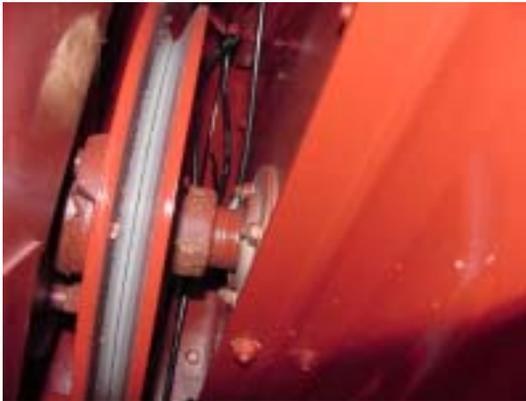
Install one # 244055, replacing grease zerk for Elevator Inner Drive Shaft. Route tubing from **Outlet 4** of Right Rear Valve.
