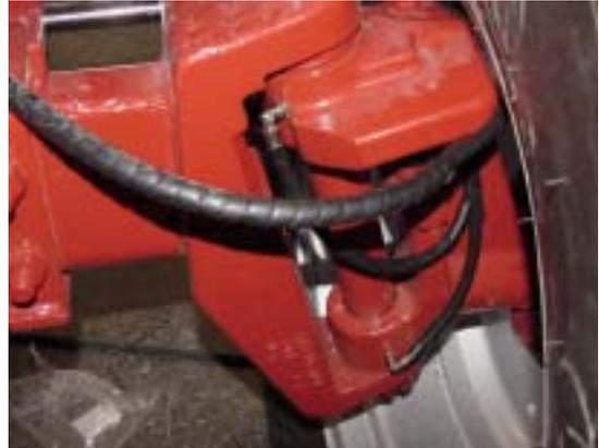
Install one # 244048 fitting, replacing grease zerk from Steering Knuckle Right Upper. This may require drilling and tapping to 1/8" NPT. Route/install tubing from **Outlet 3** of Rear Axle Valve.
