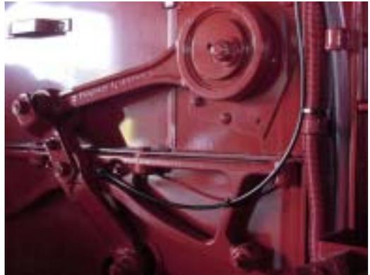
Install one # 244055 fitting, replacing grease zerk for Chaffer Hanger. Route/install tubing from **Outlet 5** of valve.
