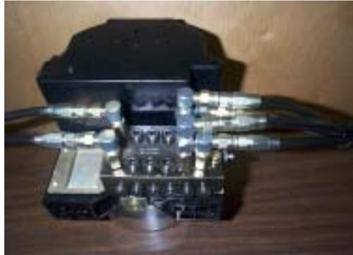
Install hose assemblies that feed the secondary valves into the primary valve located on the back of the QLS401 pump. Install hoses as described on the primary valve schematic, from the previous page. It is important to install hoses prior to the installation of the pump to the deck.
