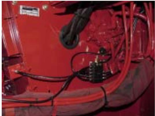
Install hose from **Outlet 9** of Primary Valve to inlet of Left Secondary Valve.
