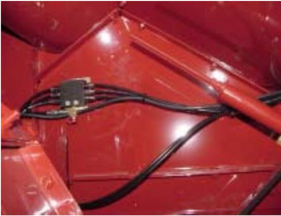
Install hose from **Outlet 10** of Primary Valve into inlet of Right Front Secondary Valve.
