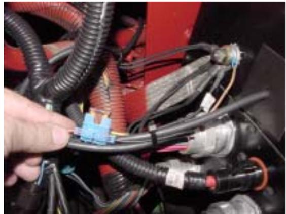
The **BLACK WIRE** is positive. This wire should be connected to the Ignition Solenoid, as shown above left, with a # 321061 terminal ring. Insert a # 241053 Fuse Holder and a # 241052 7 1/2 amp Fuse into the black positive wire as shown above.
