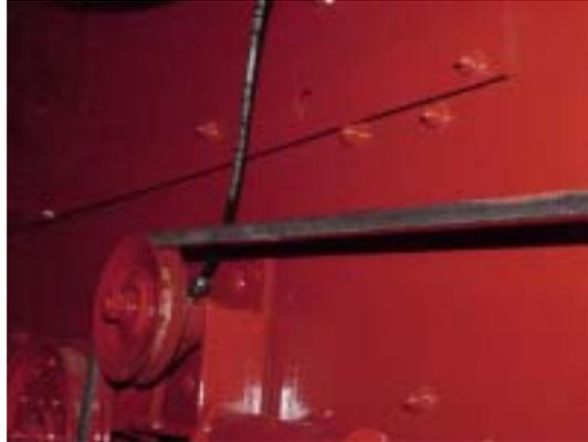
Install one # 244055 fitting, replacing grease zerk for Straw Spreader Idler Arm. Route/install tubing from **Outlet 5** of Right Rear Valve.
