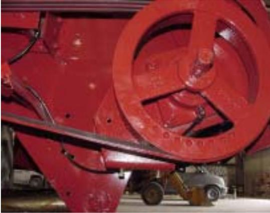
Install one of 243699, replacing grease fitting for Feeder Shaft.
