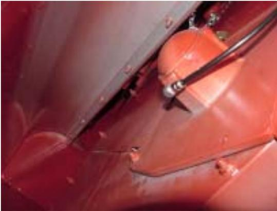
Install one of #20026 adapter and #244047 fitting, replacing grease zerk for Inclined Auger Lower Gearbox. Route/install tubing from **Outlet 1** of valve to bulkhead fittings #51055 and 13154, installed in side panel as shown in top left picture. This bulkhead fitting will require a 5/16" drilled hole. Install one 244047 into the outer end of bulkhead and a 244054 in the inner end of bulkhead. Route/install tubing (routing as shown to the right) to grease point fitting (fitting above).
