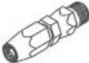
429353A1 (246002) - 1/8" NPT field installable hose coupling.....
