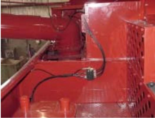
Install hose from **Outlet 2** of Primary Valve to inlet of Top Secondary Valve.
