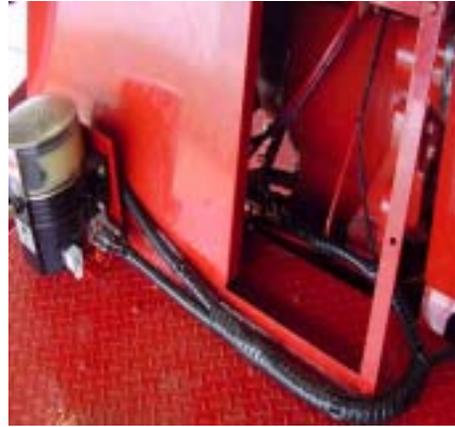
Wire routing from pump, in hose bundle on deck.
