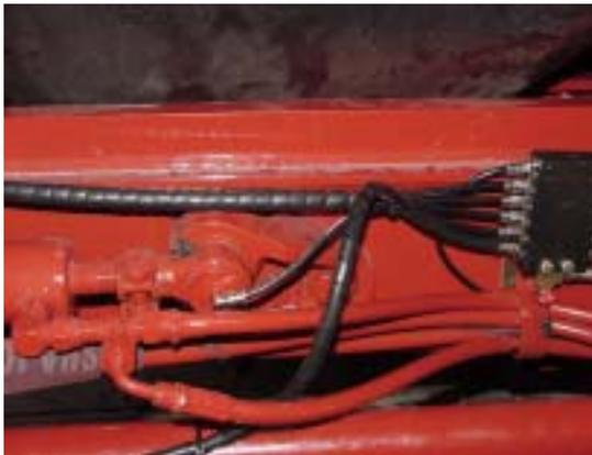
Install one # 244054 fitting, replacing grease zerk from Steering Cylinder Left Upper. Route/install tubing from **Outlet 10** of Rear Axle Valve.
