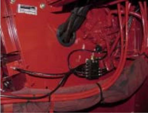
Mount Left Secondary Valve and bracket behind left front wheel, behind cab entry ladder.
