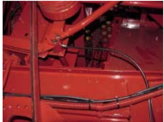
Install one # 244055 Fitting, replacing grease zerk for Straw Chopper Idler Arm. Route/install tubing from **Outlet 9** of Right Rear Valve. If option is not included, remove tubing from valve and replace with closure plug # 303174993.
