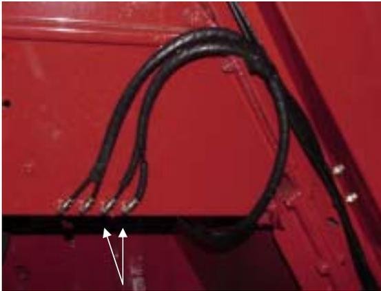
Install two # 244054 Fitting, replacing grease zerk for Steering Axle Pivot Rear Upper and Lower. Route/install tubing from **Outlets 1 and 3** of Right Rear Valve.
