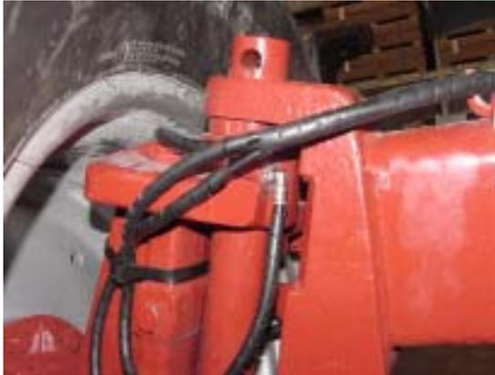
Install one # 244048 fitting, replacing grease zerk from Steering Knuckle Left Upper. This may require drilling and tapping to 1/8" NPT. Route/install tubing from **Outlet 4** of Rear Axle Valve.
