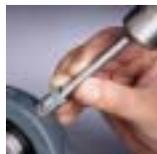
2. Tap Zerk-lock onto fitting. Position Zerk-lock on grease fitting and secure by gently tapping with hammer and staking tool.
