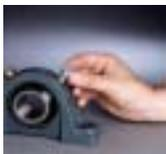
1. Place a Zerk-lock onto the grease fitting.
