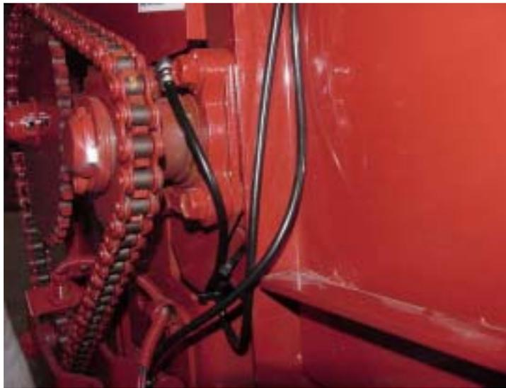
Install one # 20026 adapter and # 244047 fitting, replacing grease zerk for Rock Trap Drive. Route tubing from **Outlet 8** of valve. If option is not included, remove tubing from valve and replace with closure plug, # 303174993.
