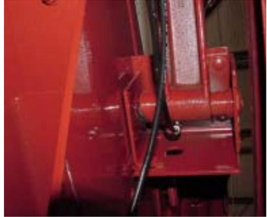
Install one of 244054, replacing grease zerker for Feeder Engage Idler Arm.
