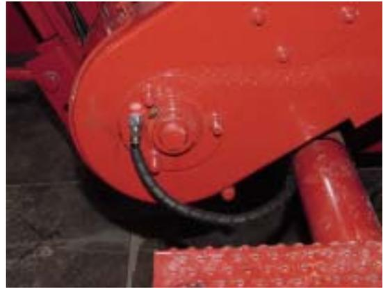
Install one # 20026 Adapter and # 244047 Fitting, replacing grease zerk for Tailings Auger Shaft Bearing. Route/install tubing from **Outlet 7** of Right Rear Valve.
