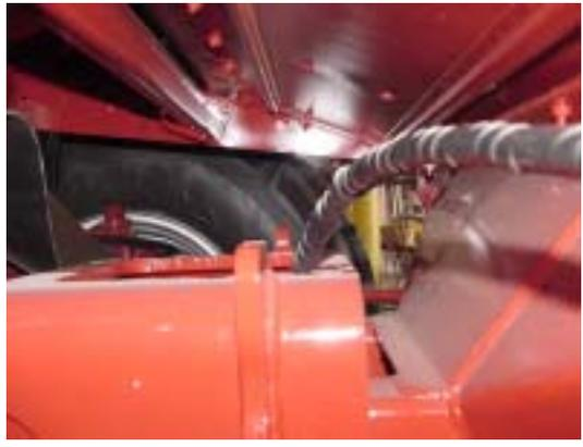
Additional line routing pictures from **Outlets 1 and 2** of the Rear Axle Valve to the right side lube bank for Steering Axle Pivot Front (Upper and Lower)
