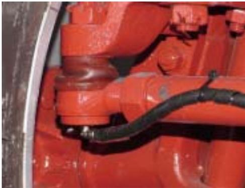
Install one of 244054 Fitting, replacing grease zerk from Tie Rod End Right. Route/install tubing from **Outlet 11** of Rear Axle Valve. Not shown with guarding. Plastic guarding is supplied in kit. Install using tie straps, also supplied in kit.
