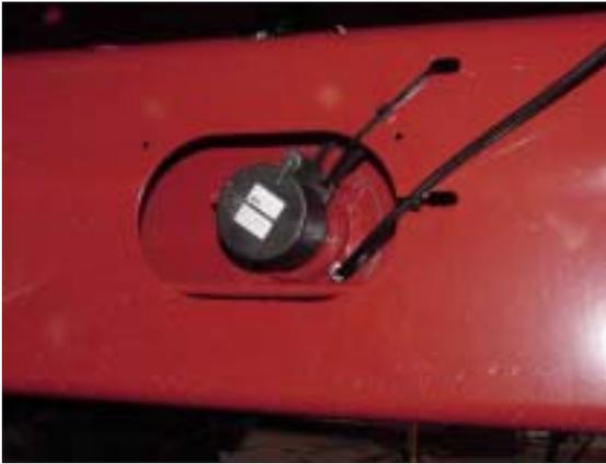
Install one #244055 fitting, replacing grease zerk for Tailings Lower Auger Shaft. Route/install tubing from **Outlet 2** of valve.
