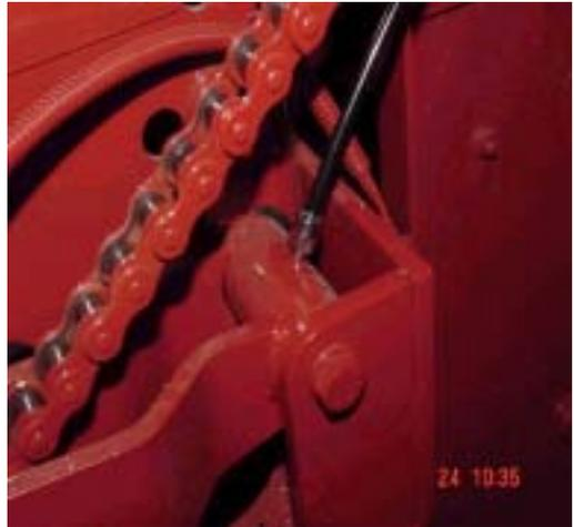
Install one # 244055 fitting, replacing grease zerk for Rock Trap Idler Gear. Route/install tubing from **Outlet 10** of valve. If option is not included, remove tubing and Quickline fitting from valve and replace with closure plug #303174993.
