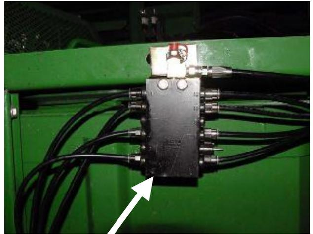
Mount Rear End Valve above chaffer indicators as shown in picture above. Use existing hardware for mounting valve bracket. Note lines should be spiral wrapped where possible for protection.
