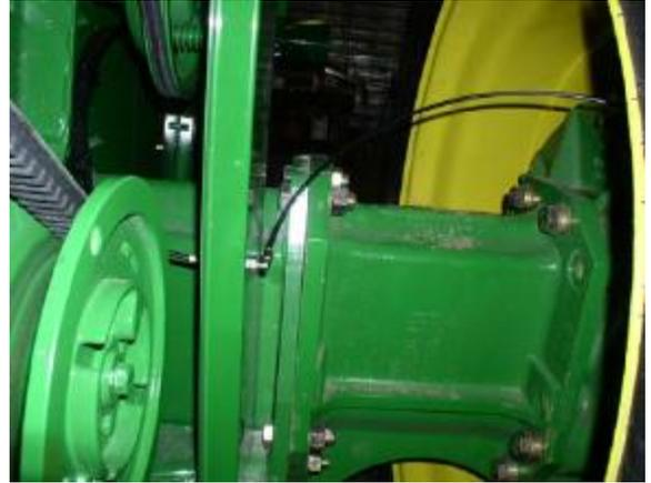
Install one # 243699, replacing grease zerk for Final Drive Outer Bearing. Route/install tubing from this fitting to bulkhead fittings # 51055 and 13154, installed in side panel as shown above. This bulkhead installation will require a 3/8" drilled hole. Install one 244047 into the inner end of bulkhead and a 243699 on the outer end of the bulkhead. Route/install tubing to outlet 1. Cut 3 ft. section from the original length.
