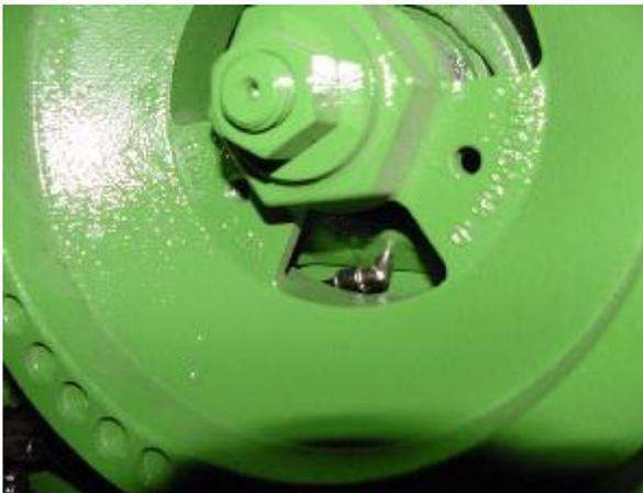
Install one # 244054 fitting, replacing grease zerk for Feed Accelerator Bearing. Rout/install tubing from outlet 2.
