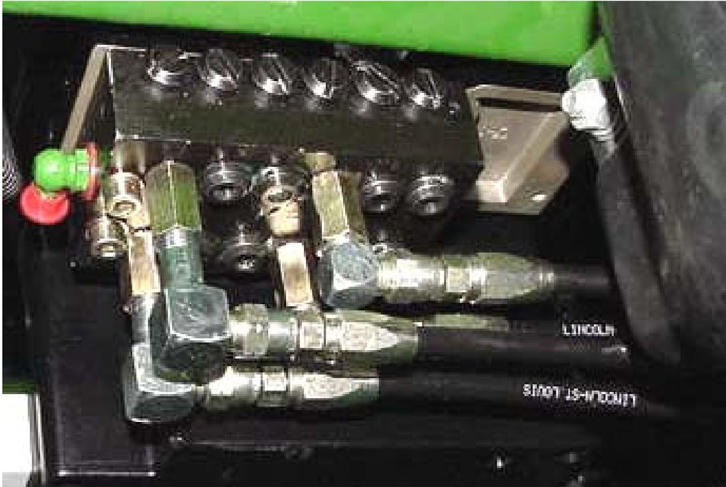
Install hose assemblies that feed the secondary valves into the primary valve located on the back of the QLS301 pump. Install hoses using locations described on the drawing (previous page). Install one end first to the appropriate secondary valve. Route hose allowing for movement and servicing if necessary. Cut hose to the required length and install 246002 hose end. Connect to fitting to the appropriate outlet of primary valve. It is easier to install the hoses prior to mounting the pump.
