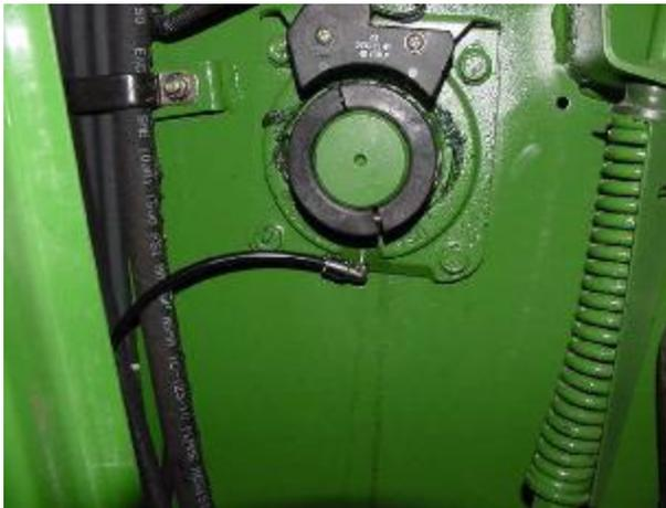
Install one 244054 fitting, replacing grease zerk for Feed Accelerator Bearing. Route/install tubing from outlet 7.
