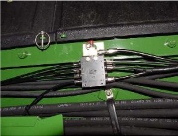
Mount Left Front Secondary Valve below separator covers as shown in picture above. Use existing hardware for mounting valve bracket.
