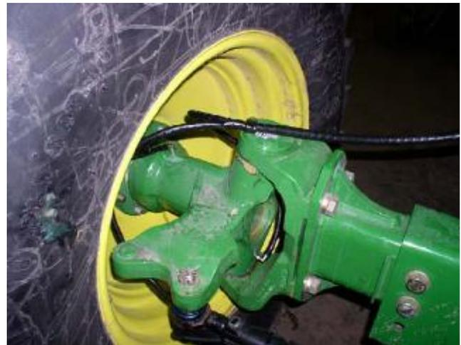
Install one 243699 fitting, replacing grease zerk for Lower Rear Axle Spindle - Left. Route/install tubing from outlet 2. Use 270931 clamp and existing hardware to attach bundle to knuckle casting.
