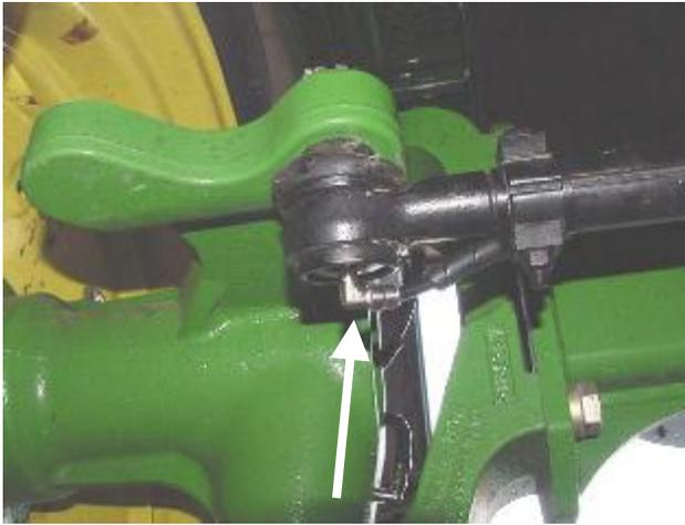
Install one 244054 fitting, replacing grease zerk for Power Steering Rod End Ball Joint. Route/install tubing from outlet 11.
