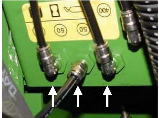
Install two 244054 fittings and one 244055 fitting, replacing grease zerk for Unloading Auger Swivel Joint (3 places). Route/install tubing from outlets 1, 2, and 5.
