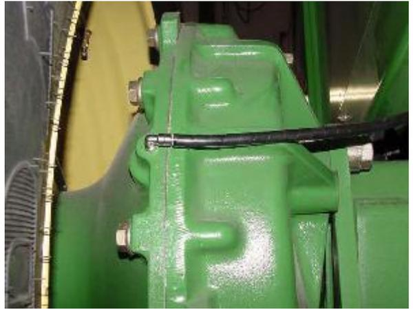
Install one 243699 fitting, replacing grease zerk for Final Drive Outer Bearing. Route/install tubing from outlet 1.
