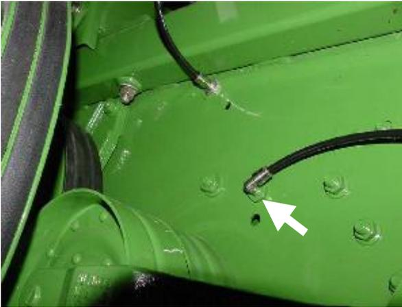
Install one 244054 fitting, replacing grease zerk for S.T.S. Separator Bearing. Route/install tubing from outlet 4.
