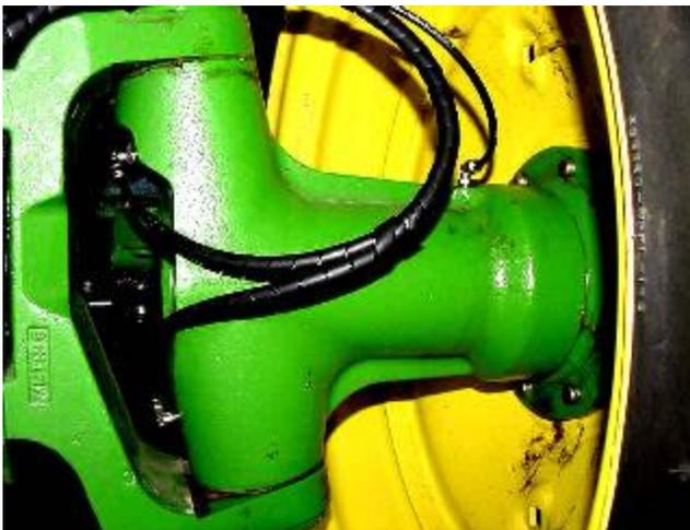
Install one 243699 fitting, replacing grease zerk for Lower Rear Axle Spindle - RightRoute/ins'. ll tubing from outlet 1. Use 270931 clamp and existing hardware to attach bundle to knuckle casting.
