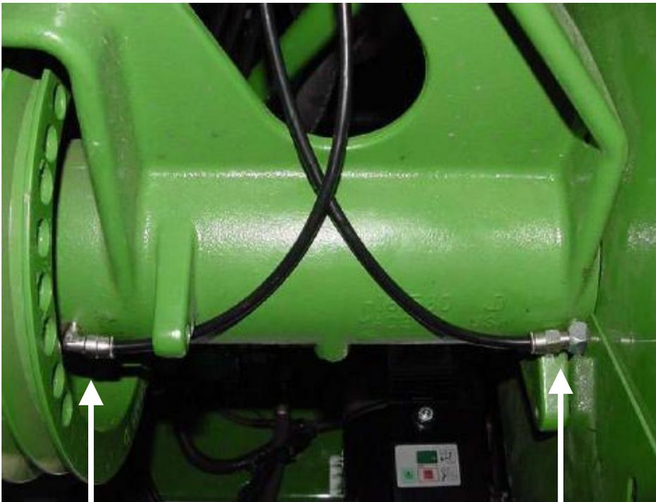
Install one 244054 fitting, replacing grease zerk for Chopper & Discharge Beater Counter Shaft. Route/install tubing from outlet 6.
