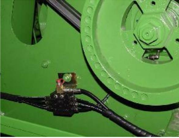
Mount Right Secondary Valve to the left of the Feed Accelerator Bearing as shown in the picture above. Use existing hardware for mounting valve bracket. Use spiral wrap to bundle/protect lines in both directions.
