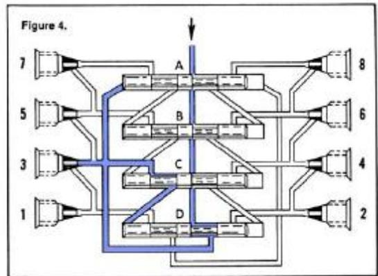
Lubricant flow shifts piston A from right to left, dispensing piston A output through Connecting passages to outlet 2. Piston A shift directs flow against right side of piston B (fig. 2).
