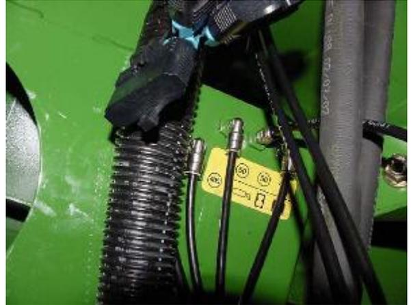
Install one 244054 fitting, replacing grease zerk for Unloader Auger Upper Gear Case. Route/install tubing from outlet 6.
