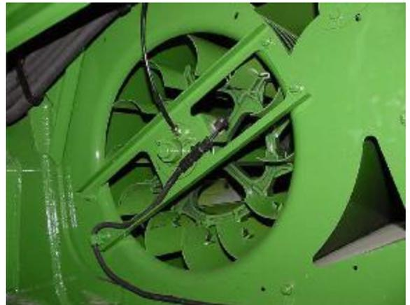
Install one 244055 fitting, replacing grease zerk for Cleaning Fan Shaft Bearing. Route/install tubing from outlet 3.
