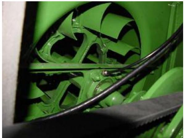
Install one 244055, replacing grease zerk for Cleaning Fan Shaft Bearing. Route/install tubing from outlet 3.
