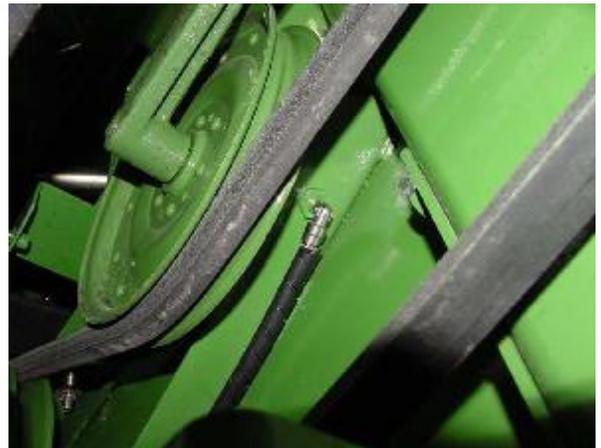
Install one 244054 fitting, replacing grease zerk for Discharge Beater Bearing. Route/install tubing from outlet 8.
