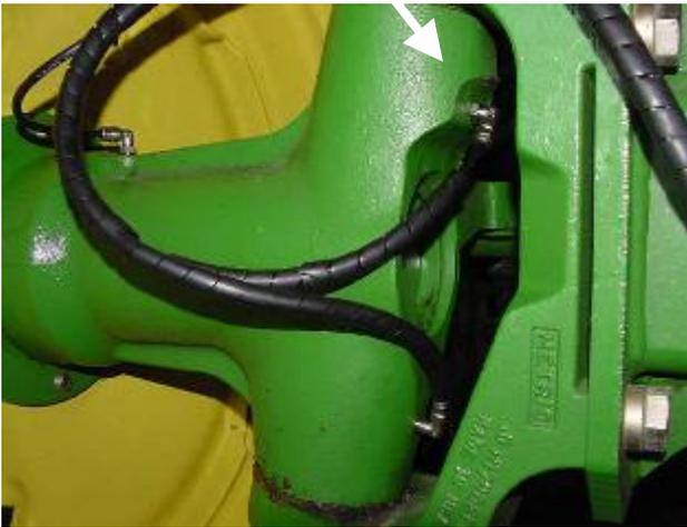
Install one 243699 fitting, replacing grease zerk for Upper Rear Axle Spindle - Left. Route/install tubing from outlet 6.
