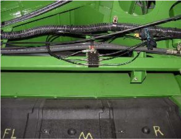
Mount Left Rear Secondary Valve above separator covers as shown in the picture above. Use existing hardware on hose clamp for mounting valve bracket. Flip the hose clamp 180 deg. For clearance.
