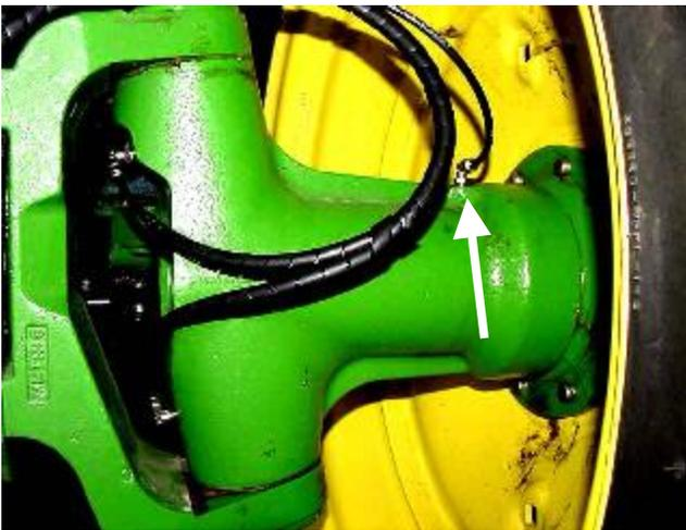
Install one 243699 fitting, replacing grease zerk for Rear Axle Spindle Bearing - Right. Route/install tubing from outlet 9.
