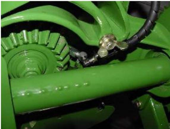
Install one 10181 and 20028 adapter and one 244048 fitting, replacing grease zerk for Unloader Auger Gear Case. Route/install tubing from outlet 2.
