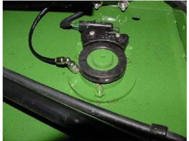
Install one 20024 adapter and one 243699 fitting, replacing grease zerk for Discharge Beater Bearing. Route/install tubing from outlet 5.
