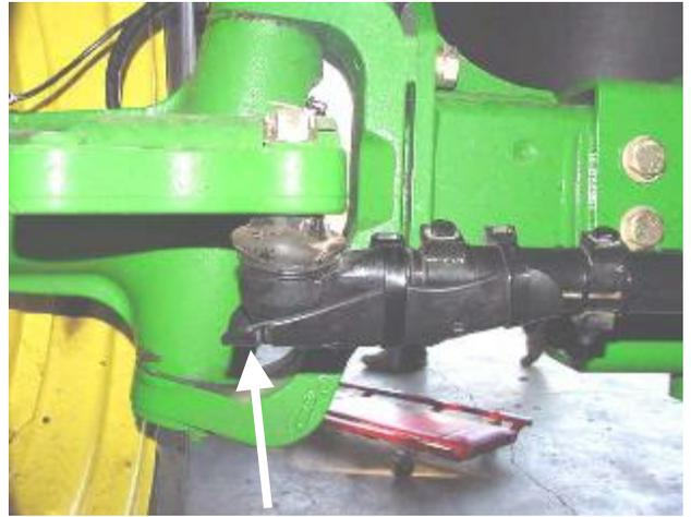
Install one 244054 fitting, replacing grease zerk for Power Steering Rod End Ball Joint - Left. Route/install tubing from outlet 12.
