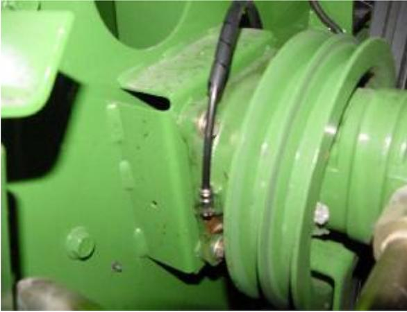
Install one 244054 fitting, replacing grease zerk for Reel Drive Pump. Route/install tubing from outlet 5.
