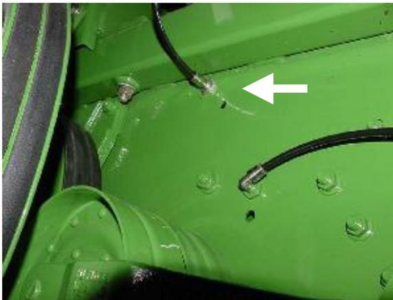
Install one 244055 fitting, replacing grease zerk for Primary Countershaft Bearing. Route/install tubing from outlet 6.
