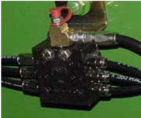
Install hose from outlet 8 of primary valve to the inlet of Right Side Secondary Valve.
