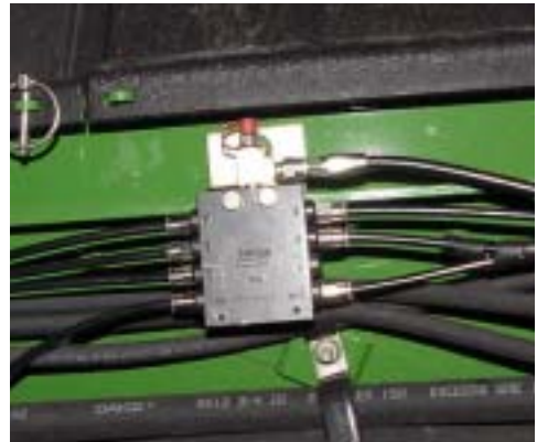
Install hose from outlet 7 of primary valve to the inlet of Left Front Secondary.
