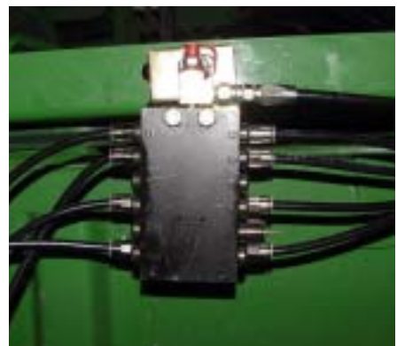
Install hose from outlet 2 of primary valve into the inlet of Rear End Secondary Valve.
