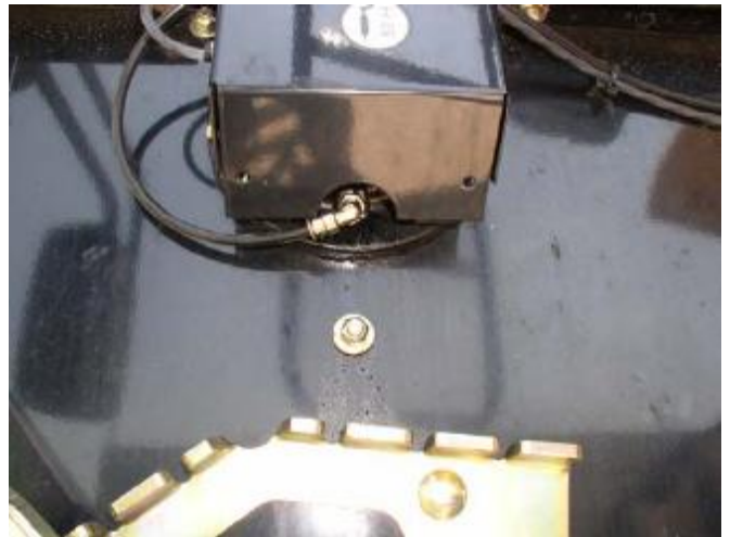
Install one #243699 fitting, replacing grease zerk for the straw chopper rotor bearing. Route/install tubing from Outlet 2 of right rear valve.
