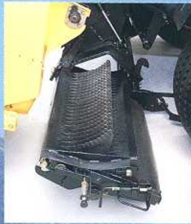
Rator cutter knives are held in this knife drawer. It slides out for simple knife inspection, sharpening or changing.
