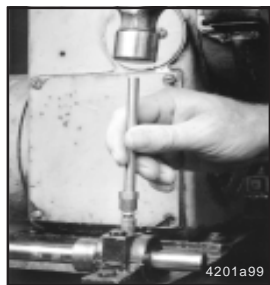
Fig. 6 - Installation of Zerk-Locks with staking tool
